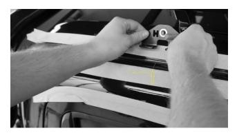
4. With a sharp knife score the vehicle paintwork either side of the mounting lug and cut down into the mastic to create a neat slot as shown in the following pictures
