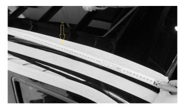
3. Mark the positions with grey lead of whiteboard marker prior removal of mastic to mount lug
