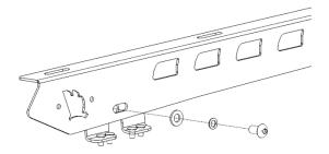
9. Fit 10mm Bolt / Flat washer/ Split washer / Strut Nuts to the top of rail.
