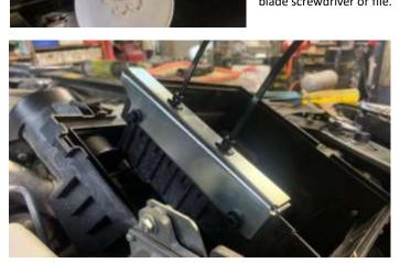
Fit the bracket with the two provided screws and insert the replacement cable ties, for holding the wiring loom.
