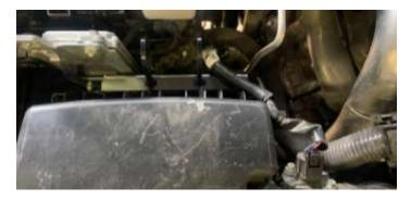
Test fit the filter and lid to the base before fitting into car. It should be a firm fit, then reinstall in to the car. Remember to tie up the wiring as best you can. If you have any issues, call us on (03) 9735 9099 or email sales@patrolapart.com.au
