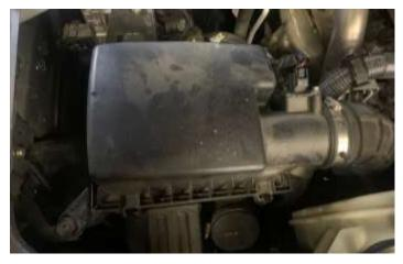
Remove lid of airbox from vehicle, then remove filter, and airbox base. (please note these instructions were done on a car fitted with Safari Snorkel, so the airbox was able to be lifted up while still fitted in car)
