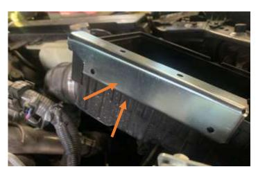
Fit bracket over the top of the two locating lugs. (you may need to remove cable ties in some models) Push bracket all the way in, and all the way up to ensure correct fitment. It is meant to be a tight fit!
