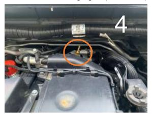
Fit Brass Breather into the Female Hose Tail through this bracket as pictured, with tail pointing up, and do up tight!
