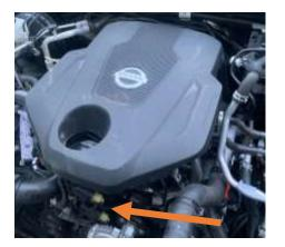
Remove Engine cover as pictured by gently lifting up to unclip the studs. The Boost Solenoids can be seen directly below the oil cap here.
